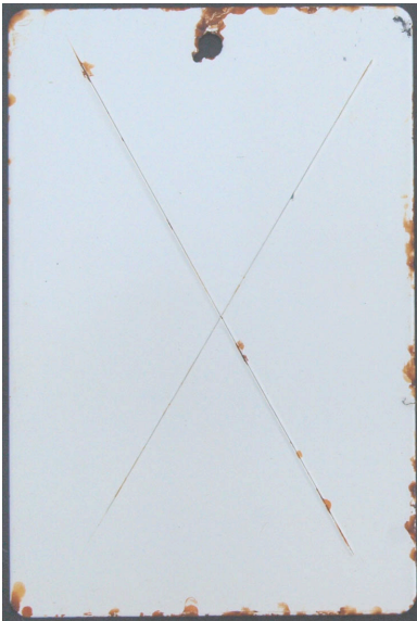
Photograph of panel after 1000hrs salt spray test
